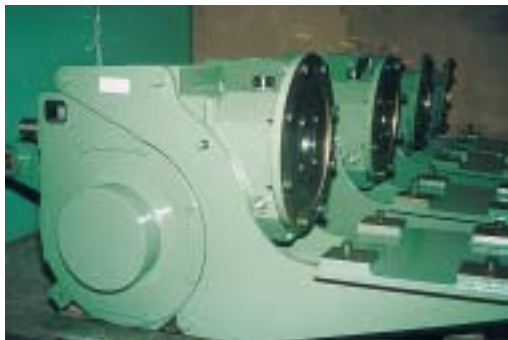
Reductores RRH-9, con palanca de inercia. RRH-9 gear box with torque arm.
