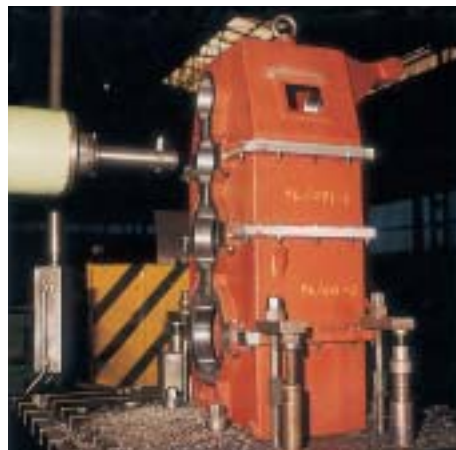
Mandrinado de carcasa para reductor. Housing boring for gear box.
